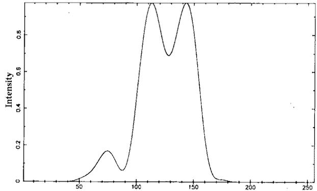
**Fig. 4.** Noise free reconstruction using the Fourier spectrum extrapolation approach. Eight complex Fourier components of the signal were retained.
